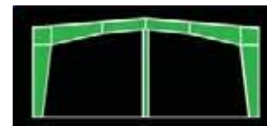
Rigid Frame Multi-Span (RF-1)
